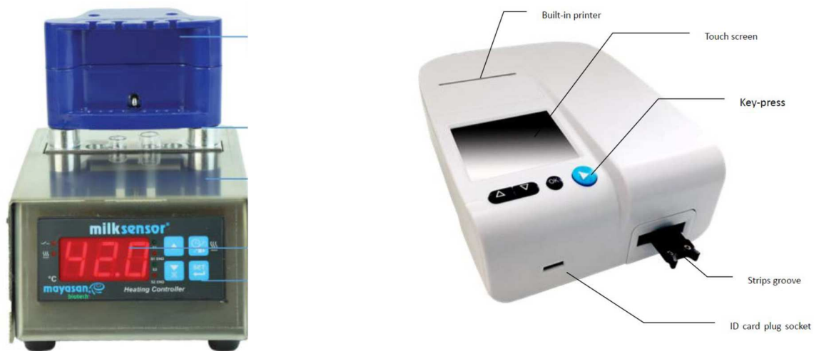
Fig. 2. Milkensor® incubator (Anon., 2021a) and reader model GIC-S1 (Anon., 2021b) for instrumental reading of the color formation on Milkensor® BT10i (β-lactams and Tetracyclines) Test Kit.
