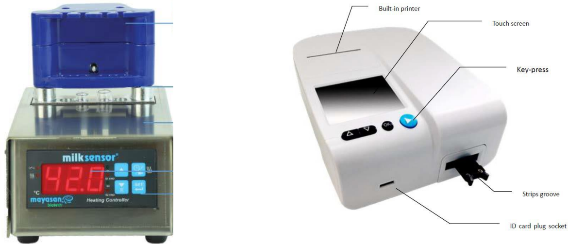
Fig. 2. Milkensor® incubator (Anon., 2021a) and reader model GIC-S1 (Anon., 2021b) for instrumental reading of the color formation on Milkensor® CBTSC10i (β-lactams & Tetracyclines, Streptomycin & Chloramphenicol) Test Kit.
